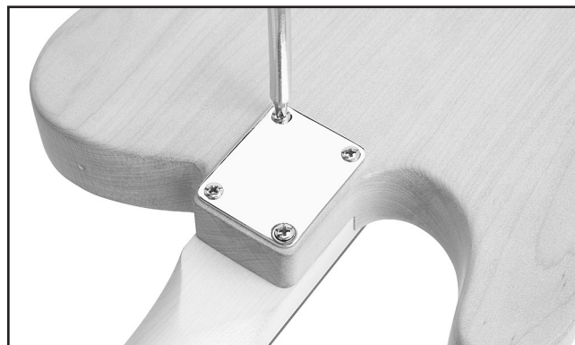
Figure 12. Fastening neck to body.
